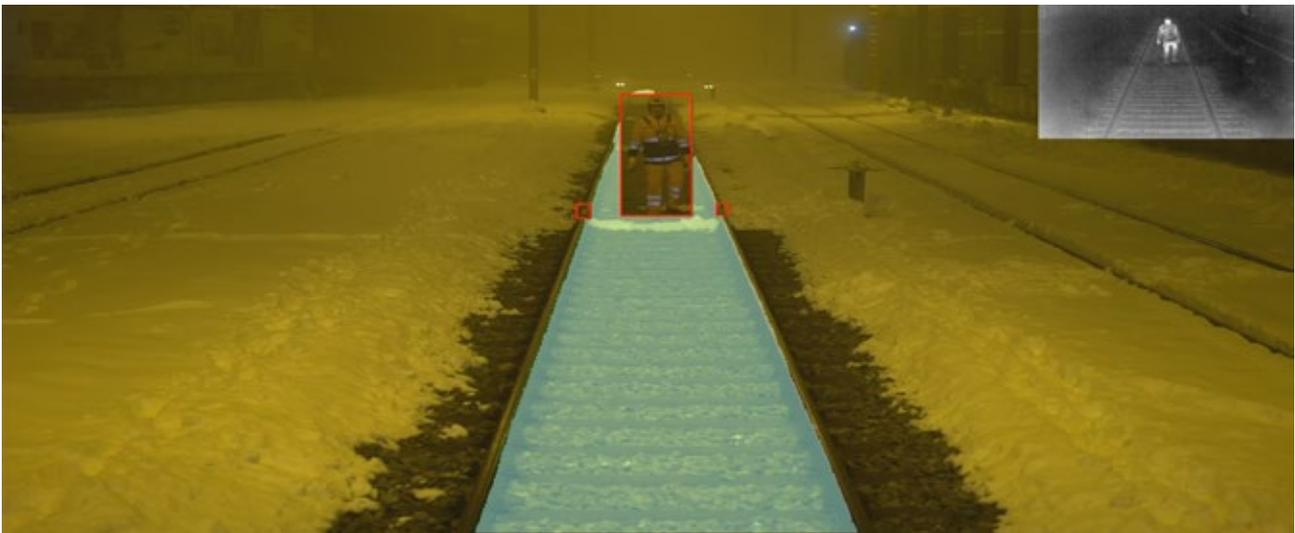
*Human & braking shoes detection at night and in harsh weather conditions*
